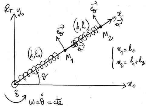
$$\text{soit } \ddot{l}_1 + \omega^2 (K-1) l_1 = \omega^2 K l_2 \quad (1')$$
