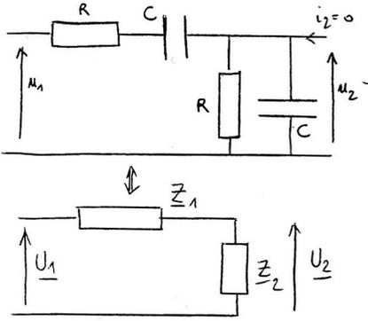
$H = \frac{1}{1 + 1 + jRC\omega + \frac{1}{jRC\omega} + 1} = \frac{1}{3 + j(RC\omega - \frac{1}{RC\omega})} \Rightarrow H = \frac{1/3}{1 + j\frac{1}{3}(RC\omega - \frac{1}{RC\omega})}$
