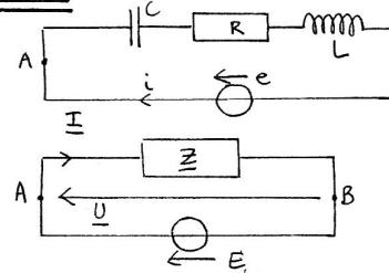
$$\underline{Z} = \frac{1}{j\omega C} + R + jL\omega = R + j(L\omega - \frac{1}{C\omega})$$
