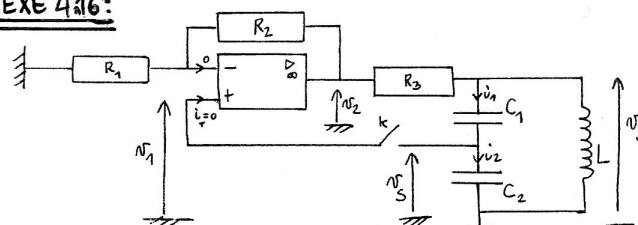
$$(1) \frac{\underline{V}_2}{\underline{V}_1} = \frac{R_1 + R_2}{R_1}$$
