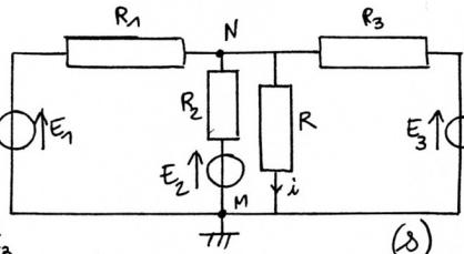
$$\text{d'où } V_N \left( \frac{1}{R_1} + \frac{1}{R_2} + \frac{1}{R} + \frac{1}{R_3} \right) = \frac{E_1}{R_1} + \frac{E_2}{R_2} + \frac{E_3}{R_3} \quad (1)$$
