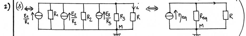
$$\text{avec } \left\{ \begin{array}{l} E_{eq} = \frac{E_1 + E_2 + E_3}{R_1 + R_2 + R_3} \\ \frac{1}{Req} = \frac{1}{R_1} + \frac{1}{R_2} + \frac{1}{R_3} \end{array} \right.$$
